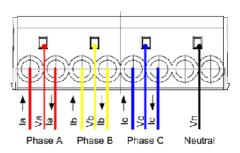
For an installation > 70 kWc, you must use Current Transformers (CTs) to measure the current. The transformation ratio must be specified with the order.
